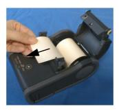
When installing the label paper vertically: Set the new roll paper in the inside of the roll paper cover. Pull the leading edge of the roll paper. Align the left edge of the roll paper with the edge of the cover.
